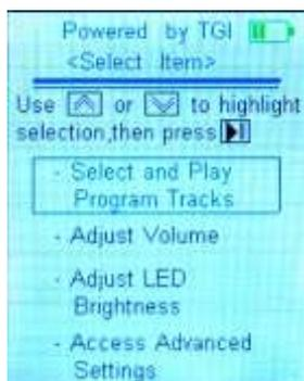
First Step: Power up the MASTER KEY – Hold the center button until the "Select Item" screen at the left appears. Note that there are four options. An option can be selected by using the up or down arrows on the control wheel to move the selection box. Pressing the center button once will display the corresponding screen. NOTE: At any time while making your selections should you wish to go back to the previous screen, press the up arrow.
