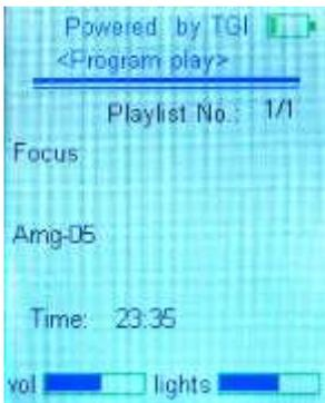
Note that the Topic and Track ID are shown, along with the time remaining in the program. The settings for earphone volume and TGiWear brightness are also shown. While the program is playing the right or left arrows will increase or decrease the volume respectively, and up or down arrows will increase or decrease the TGiWear brightness level.
